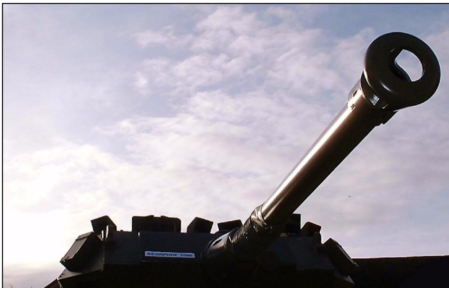
90 mm MAIN GUN UPGRADE IN STANDARD SCORPION TURRET
