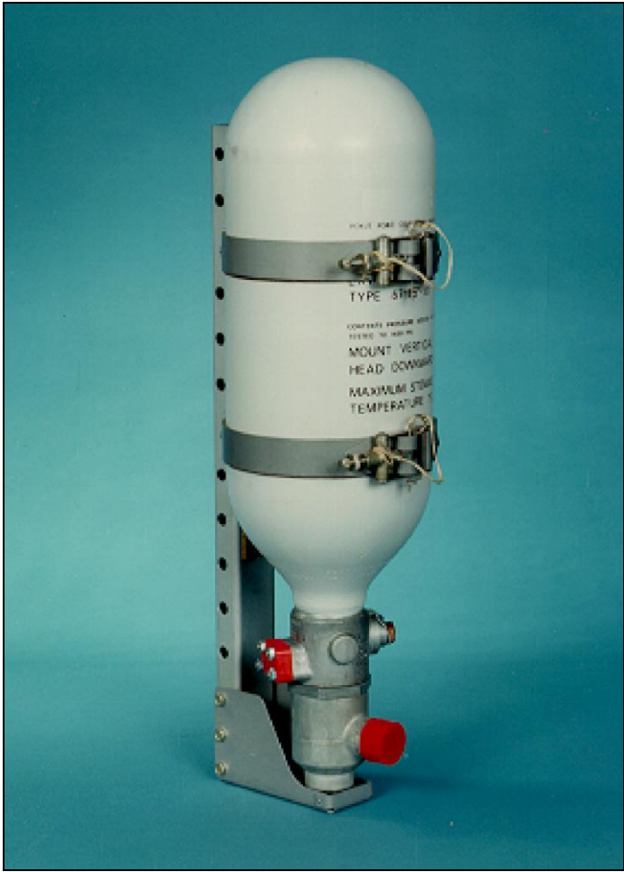
TYPICAL ENGINE BAY EXTINGUISHER BOTTLE
