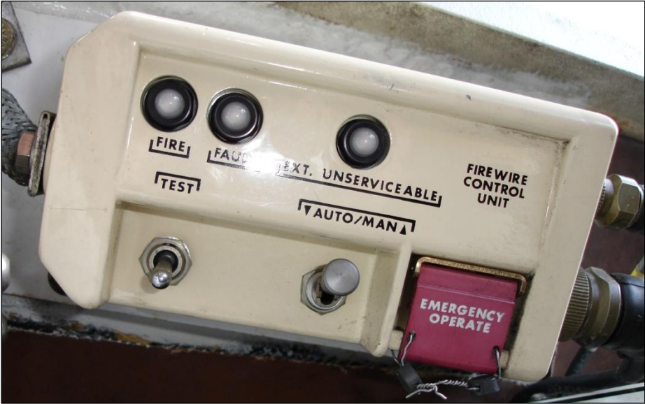
TYPICAL ENGINE BAY CONTROL UNIT
